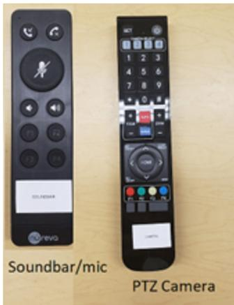
The Nureva remote can be used to change the volume (this can be done on the computer as well). The camera remote can be used to zoom in and out, and pan/tilt/zoom to point the camera where you would like it. You can also save presets so that the camera can snap to specific pre-determined locations in the classroom.
